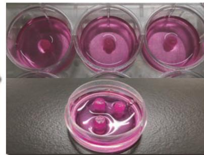
**3** Complete by adding liquid medium after cell attachment. Multiple sponges can also be cultured in a 6 well or 35 mm dish.
