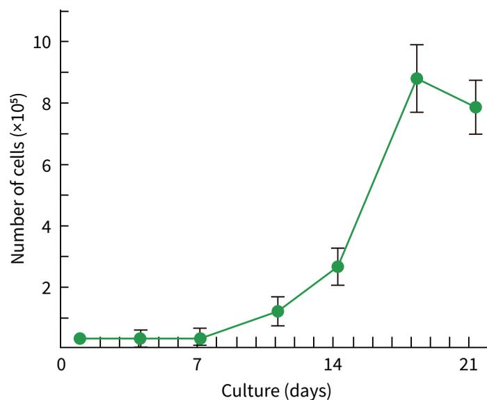
**3D Honeycomb Boosted** has pores concentrated around 200~250 µm, and a high-density 3D culture is enable. After seeding  $1 \times 10^4$  cells, it was possible to culture up to about  $10^6$  cells after 18 days. (Based on in-house data.)
