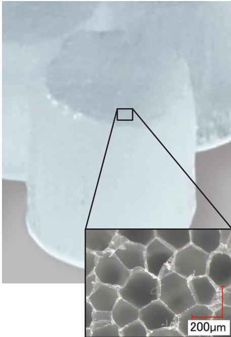
Koken's AteloCell® **3D Honeycomb Boosted** (KKN-3D-HCB) is designed as a scaffold for high density 3D cell culture/cell transplantation.
