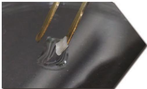
**1** Compress the sponge with flat-tipped tweezers to remove PBS and transfer to a plate or dish.
