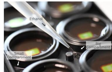
Figure 3: Filling Compartments between Wells with 70% Ethanol
