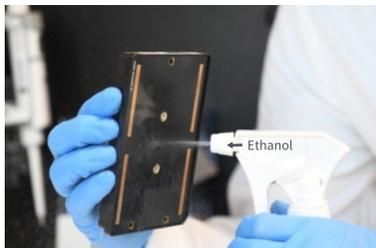
Figure 1: Spraying MaxTwo Multi-Well Plate with 70% Ethanol
