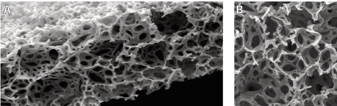
Scanning electron microscope image of Alvetex Scaffold, to highlight its porous structure. **A:** a 200 µm thick Alvetex Scaffold disc. **B:** Close up of Alvetex Scaffold voids with dimensions of approximately 42 µm in diameter and interconnects of approximately 13 µm in diameter.
