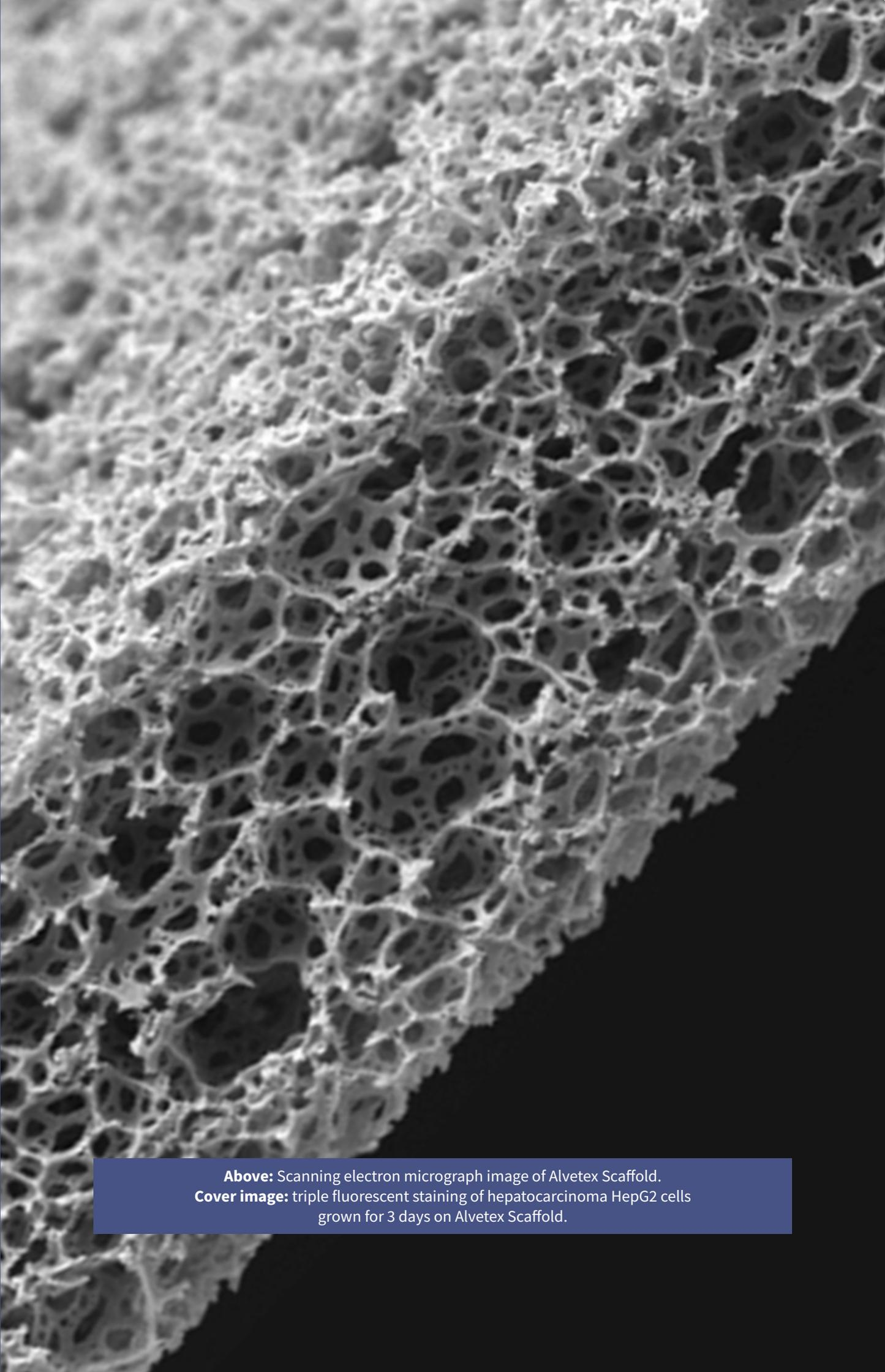
**Above:** Scanning electron micrograph image of Alvetex Scaffold.
