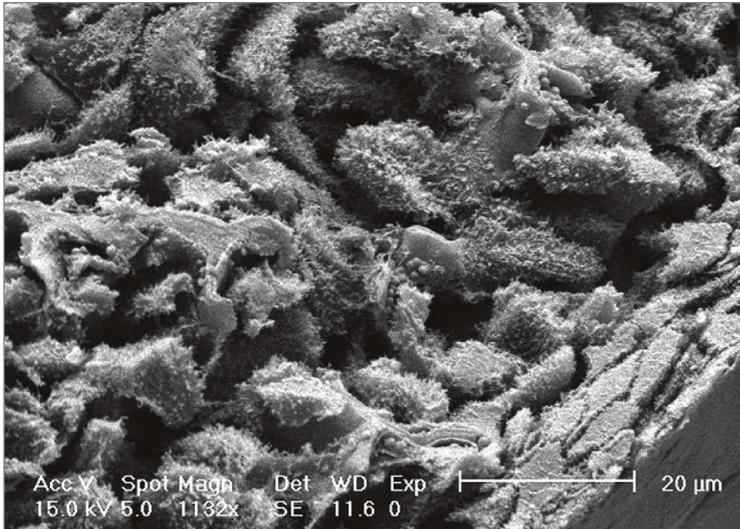
Visualization of the structure of 3D cultures in Alvetex Scaffold is made possible using scanning electron microscopy (SEM). Samples are prepared in the same manner as would normally be used for tissues. In this example, skin, cells have penetrated throughout the scaffold and some have stratified on the surface (lower right corner).
