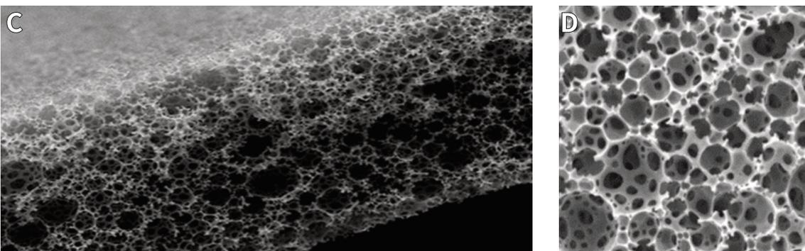
Scanning electron microscope image of Alvetex Strata. **C:** a 200 µm thick Alvetex Strata disc. **D:** Close up of Alvetex Strata voids with dimensions of approximately 15 µm in diameter and interconnects of approximately 5 µm in diameter.
